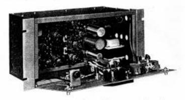
The Level Devil front panel hinges down for fast access to tubes and controls. As controls once adjusted are seldom changed, this feature prevents accidental changing of the important automatic gain control functions. The controls accessible with front panel closed include an-off switch, pilot light and fuse.
